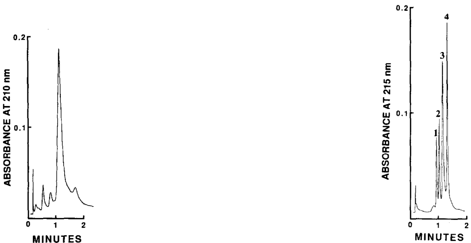
Fig. 6. Ion-exchange chromatography of commercial ovalbumin. Column, micropellicular PEI ( 30 \times 4.6 mm I.D.). The sample components were eluted by a linear increase of NaCl from 0 to 0.5 M in 5 min with 25 mM phosphate buffer (pH 7.5). The main peak represents ovalbumin and its glycosylated/phosphorylated conformers are shown by the minor peaks. Flow-rate, 2 ml/min; temperature, 70°C.
